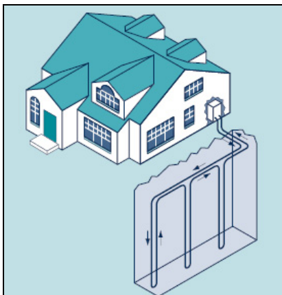
Figure 9: Geothermal heat pump with vertical loop
